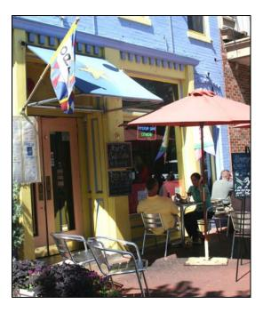
Shed-style awnings and canopies are generally the most appropriate form for a flat-topped opening. Awnings and canopies should only be attached to a building in a manner that does not cause permanent damage, generally not through masonry. Awnings and canopies should have a minimum clearance height of 8'.
